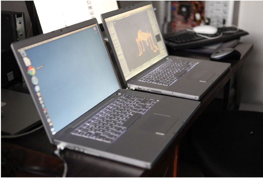
MacBook Pro version 1.1 from 2006 and version 2.2. The latter has a 3-gigabyte memory limit.
